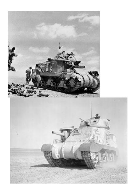
The Grant was first received by the British in 1941 and the Lee in 1942. The Grant was built to British specifications and the Lee was the standard version of the Tank. At the time it gave the British an advantage against the German tanks as it's armour was superior and the hull 75mm gun could deal with
