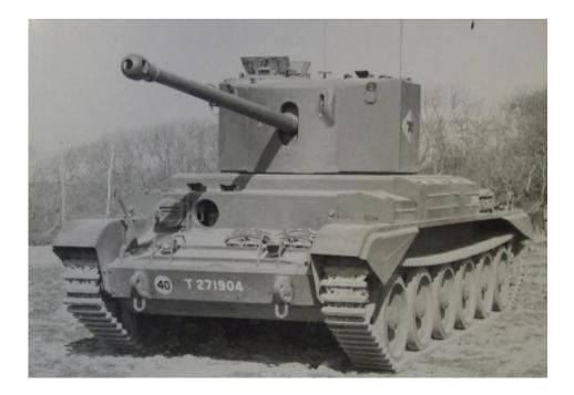
The Challenger was the first British tank to mount the 17 pounder gun and was essentially a modified Cromwell with a larger turret. Due to the large turret size the vehicle was very top heavy but it retained most of the Cromwells high speed and agility. Only around 200 of the vehicles were ordered with 197 being completed by the time war ended in Europe. Additional 25mm armour plates were welded to the front of the vehicle to provide extra protection.
