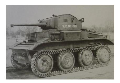
The Tetrarch was a light tank designed by Vickers-Armstrong, it was very fast but armour was extremely thin. Production was very limited but increased slightly when it was found that the Tetrarch could be carried by gliders to support airborne troops.
